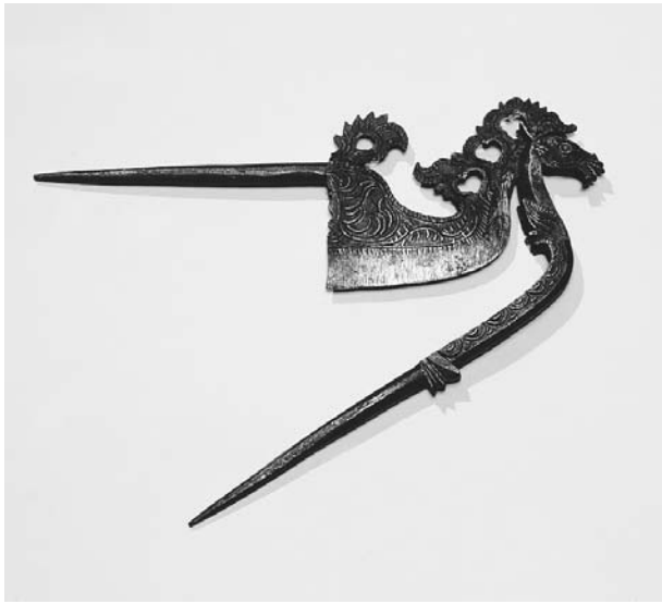
Betel nut sheller, Sri Lanka, nineteenth century. Wrought iron. The sharp blade cracks open the nut while the pointed handles serve as nut picks. ROUGHWOOD COLLECTION. PHOTO CHEW & COMPANY.
